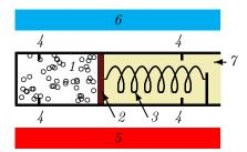
and maximum volumes occupied by the working body, figure 1. In the ultimate states of maximum compression and extension of the spring its potential energy is maximum. In the intermediate state where the spring is relaxed, its potential energy is zero, while the kinetic energy of the working body and the piston is not.
